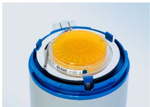
Figure 4: 400x0.7 mm contact plate after sampling 1000 L ambient air with MAS-100 NT® and contact plate adapter: The regular impactation pattern demonstrates homogeneous air impact over the complete agar surface
