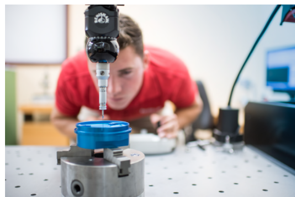
Figure 6: Quality control of a sampling base. State of the art risk-based test plans assure that production lots remain within specifications.
