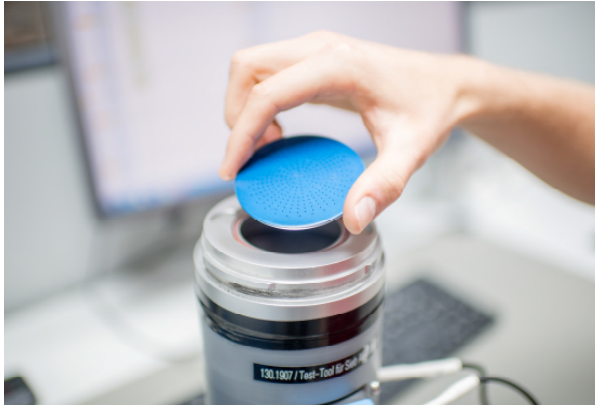
Figure 7: An aluminium sieve is tested for airflow as the anodization has an influence on the hole diameter and therefore on impaction speed.
