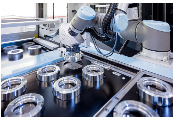
Figure 5: Perforated lids in production. Mounting robots in combination with the most modern machining tools produce parts within very narrow specifications. Picture courtesy Femron AG ( www.femron.ch )
