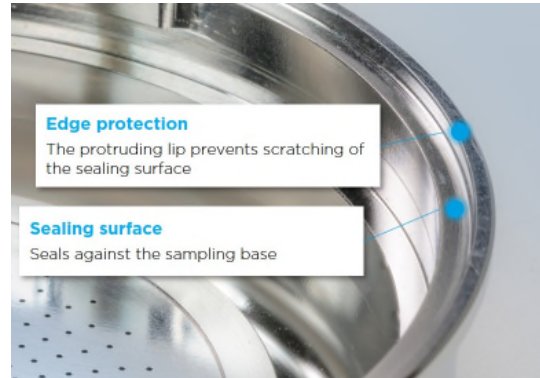
Figure 4: Stainless steel perforated lid (upside down). The edge protection prevents scratching of the sealing surface which would lead to aspirating air through the gap.
