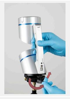
The mounted adapter plate can remain on the instrument, it fits in the hygiene inspection case.
