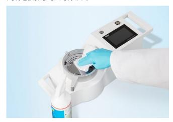
Optionally, the base for nutrient plates can be removed for autoclaving. In this case make sure to protect the sampling head base with the dust cover. While removing the nutrient plate holder, take care not to touch nor damage the instrument filter, if in doubt, it is recommended to replace the filter (see chapter 5.3 «Replacing the instrument filter»).
