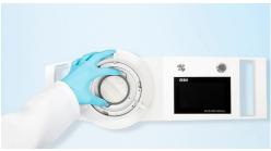
Insert a fresh HEPA H13 filter (see chapter 2.6 «Accessories for MAS-100 Atmos»). Pay attention not to touch the filter membrane because of risk of damaging it. Carefully apply the filter cover and attach it with the three screws.
