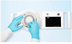
Open the filter cover with a screwdriver. Remove the underlying filter carefully.
