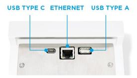
To prevent the ports from dust, the less frequently used Ethernet and USB type A interfaces are protected with protecting caps.
